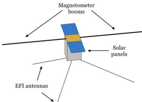
*Figure 3: smallsat sketch showing accommodation of field instruments. Particle instruments will be accommodated on the sides or edges of the smallsats to have an unobstructed lateral view.*
